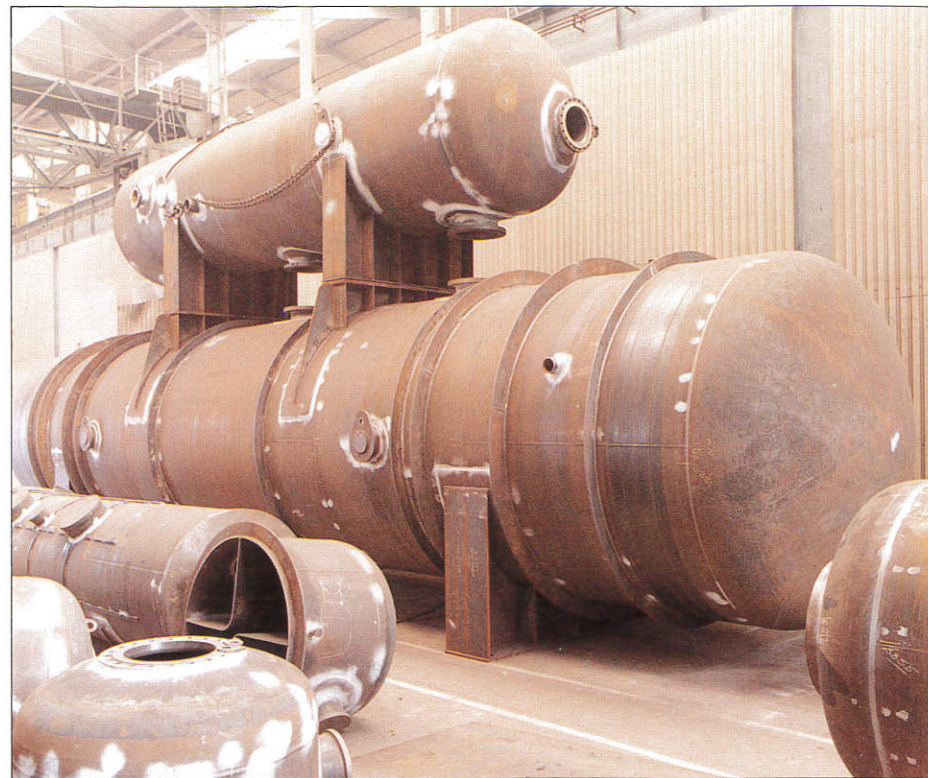
1 Trial erection in our works of a deareator vessel and storage tank. Part of a two set order shipped to Hong Kong.
